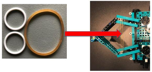
Furthermore, the pen should move smoothly over the paper. The height off he pen tip should be adjusted in a way to just barely touch the paper when the pen is in the lowered position. When the pen is pressed too hard tot he paper, the friction may prevent the pen from reaching the programmed positions.
